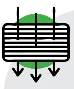
Regular (once every 3 to 4 weeks) cleaning of air-conditioner filters ensures that more cool air will be allowed to flow out thus reducing the need to reduce the temperature and/or increase the fan speed.
