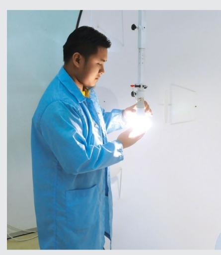
A lab technician at the photometry test facility placing a bulb into the integrating sphere which measures the light characteristics of lamps.
